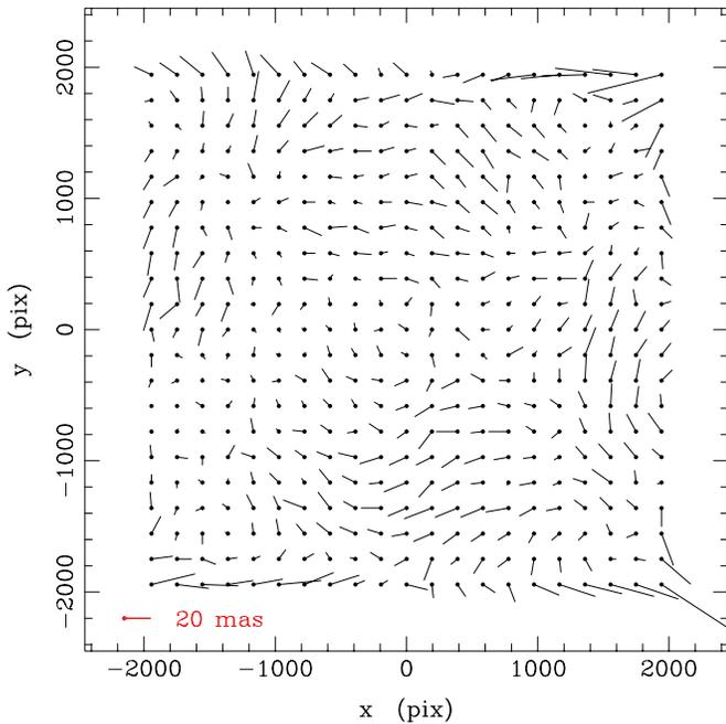
**Figure 2.** Field-distortion correction mask for the PV CCD/filter combination. The mask was derived by stacking residuals of PV frames reduced into UCAC2 positions. The scale of the vectors is as indicated in the lower left.
